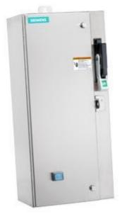
Non-reversing motor starter Size 1 Three phase full voltage Amb compensate bimetal OLrelay Contactor amp rating 27Amp 380-440/440-480V 50/60HZ coil Combination type 60Amp fusible disconnect 60Amp / 250V fuse clip Encl NEMA type 4X 304 S-steel Water/dust tight non-corrosive Standard width enclosure
