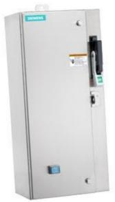
Non-reversing motor starter Size 1 Three phase full voltage Amb compensate bimetal OLrelay Contactor amp rating 27Amp 24VAC 50-60HZ coil Combination type 60Amp fusible disconnect 60Amp / 250V fuse clip Encl NEMA type 4X 304 S-steel Water/dust tight non-corrosive Standard width enclosure
