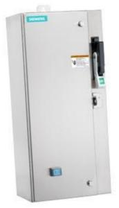
Non-reversing motor starter Size 1 Three phase full voltage Amb compensate bimetal OLrelay Contactor amp rating 27Amp 240VAC 50HZ / 277VAC 60HZ coil Combination type 30Amp fusible disconnect 30 Amp /600V fuse clip Encl NEMA type 4X 304 S-steel Water/dust tight non-corrosive Standard width enclosure
