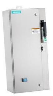
Non-reversing motor starter Size 1 Three phase full voltage Amb compensate bimetal OLrelay Contactor amp rating 27Amp 24Vdc coil Combination type 30Amp fusible disconnect 30Amp / 250V fuse clip Encl NEMA type 4X 304 S-steel Water/dust tight non-corrosive Standard width enclosure
