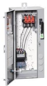
Non-reversing motor starter, Size 1, Three phase full voltage, Solid-state overload relay, OLRelay amp range 3-12a, 190 220/220 240V 50/60HZ coil, Combination type, 30Amp non-fusible disconnect Enclosure NEMA type 4/12, Water/dust tight for outdoors, Standard width enclosure
