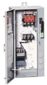
Non-reversing motor starter Size 1 Three phase full voltage Solidstate overload relay OLRelay amp range 3-12A 24Vdc coil Combination type 30Amp fusible disconnect 30Amp / 250V fuse clip Enclosure NEMA type 4/12 Water/dust tight weather proof Standard width enclosure
