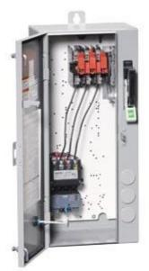
Non-reversing motor starter, Size 1, Three phase full voltage, Solidstate overload relay, OLRelay amp range 5.5-22a, 208VAC 60HZ coil, Combination type, 30Amp non-fusible disconnect Enclosure NEMA type 4/12, Water/dust tight for outdoors, Standard width enclosure
