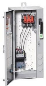
Non-reversing motor starter, Size 1, Three phase full voltage, Solidstate overload relay, OLRelay amp range 5.5-22a, 110V 50HZ / 120V 60HZ coil, Combination type, 30Amp non-fusible disconnect Enclosure NEMA type 4/12, Water/dust tight for outdoors, Standard width enclosure
