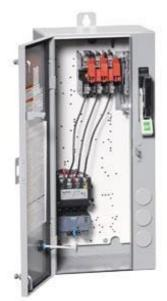
Non-reversing motor starter, Size 1, Three phase full voltage, Solid-state overload relay, OLRelay amp range 5.5-22a, 380 440/440 480V 50/60HZ coil, Combination type, 30Amp non-fusible disconnect Enclosure NEMA type 4/12, Water/dust tight for outdoors, Standard width enclosure
