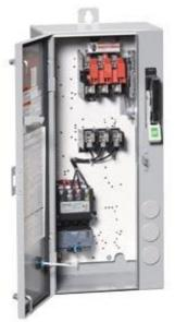
Non-reversing motor starter Size 1 Three phase full voltage Solidstate overload relay OLRelay amp range 5.5-22A 24Vdc coil Combination type 30Amp fusible disconnect 30Amp / 250V fuse clip Enclosure NEMA type 4/12 Water/dust tight weather proof Standard width enclosure
