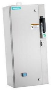
Non-reversing motor starter Size 1 Three phase full voltage Solidstate overload relay OLRelay amp range 5.5-22A 110VAC 50HZ / 120VAC 60HZ coil Combination type 30Amp fusible disconnect 30Amp / 250V fuse clip Encl NEMA type 4X 304 S-steel Water/dust tight non-corrosive Standard width enclosure
