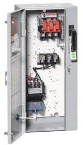
Non-reversing motor starter, Size 1, Three phase full voltage, Solidstate overload relay, OLRelay amp range 10-40a, 190 220/220 240V 50/60HZ coil, Combination type, 30Amp fusible disconnect 30 Amp /250V fuse clip, Enclosure NEMA type 1, Indoor general purpose use, Standard width enclosure
