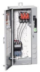
Non-reversing motor starter, Size 1, Three phase full voltage, Solidstate overload relay, OLRelay amp range 10-40a, 380 440/440 480V 50/60HZ coil, Combination type, 60Amp non-fused disconnect Enclosure NEMA type 4/12, Water/dust tight for outdoors, Standard width enclosure
