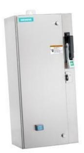
Non-reversing motor starter, Size 1, Three phase full voltage, Solidstate overload relay, OLRelay amp range 10-40a, 24VAC 50-60HZ coil, Combination type, 30Amp fusible disconnect 30 Amp /250V fuse clip, Encl NEMA type 4X 304 S-steel Water/dust tight noncorrosive, Standard width enclosure
