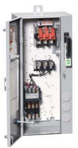
Non-reversing motor starter Size 1 3/4 Three phase full voltage Amb compensate bimetal OLrelay Contactor amp rating 40Amp Combination type 60Amp fusible disconnect 60Amp / 600V fuse clip Enclosure NEMA type 4/12 Water/dust tight weather proof Standard width enclosure
