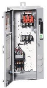
Non-reversing motor starter Size 1 3/4 Three phase full voltage Amb compensate bimetal OLrelay Contactor amp rating 40Amp Combination type 60Amp fusible disconnect 60Amp / 600V fuse clip Enclosure NEMA type 4/12 Water/dust tight weather proof Standard width enclosure
