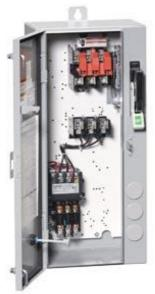
Non-reversing motor starter Size 1 3/4 Three phase full voltage Amb compensate bimetal OLrelay Contactor amp rating 40Amp 24VAC 50-60HZ coil Combination type 60Amp fusible disconnect 60Amp / 600V fuse clip Enclosure NEMA type 4/12 Water/dust tight weather proof Standard width enclosure
