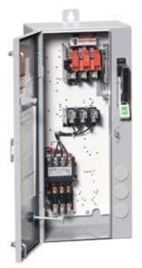
Non-reversing motor starter Size 1 3/4 Three phase full voltage Amb compensate bimetal OLrelay Contactor amp rating 40Amp 240VAC 50HZ / 277VAC 60HZ coil Combination type 60Amp fusible disconnect 60Amp / 600V fuse clip Enclosure NEMA type 4/12 Water/dust tight weather proof Standard width enclosure
