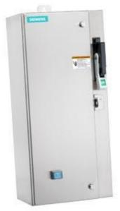
Non-reversing motor starter Size 1 3/4 Three phase full voltage Amb compensate bimetal OLrelay Contactor amp rating 40Amp 380-440/440-480V 50/60HZ coil Combination type 60Amp fusible disconnect 60Amp / 600V fuse clip Encl NEMA type 4X 304 S-steel Water/dust tight non-corrosive Standard width enclosure
