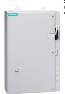
Non-reversing motor starter, Size 1 3/4, Three phase full voltage, Solid-state overload relay, OLRelay amp range 10-40a, 110 120/220 240VAC 60HZ coil, Combination type, 60Amp non-fused disconnect Enclosure NEMA type 4/12, Water/dust tight for outdoors, Extra-wide enclosure
