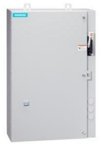
Non-reversing motor starter, Size 1 3/4, Three phase full voltage, Solid-state overload relay, OLRelay amp range 10-40a, 220 240/440 480VAC 60HZ coil, Combination type, 60Amp non-fused disconnect Enclosure NEMA type 4/12, Water/dust tight for outdoors, Extra-wide enclosure
