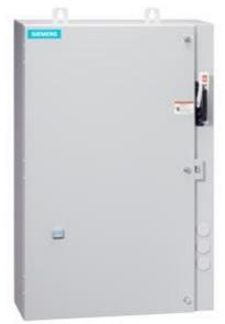
Non-reversing motor starter, Size 1 3/4, Three phase full voltage, Solid-state overload relay, OLRelay amp range 10-40a, 208VAC 60HZ coil, Combination type, 60Amp non-fused disconnect Enclosure NEMA type 4/12, Water/dust tight for outdoors, Extra-wide enclosure
