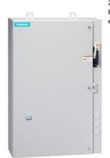
Non-reversing motor starter, Size 1 3/4, Three phase full voltage, Solid-state overload relay, OLRelay amp range 10-40a, 190 220/220 240V 50/60HZ coil, Combination type, 60Amp non-fused disconnect Enclosure NEMA type 4/12, Water/dust tight for outdoors, Extra-wide enclosure
