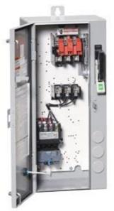
Non-reversing motor starter Size 1 3/4 Three phase full voltage Solid-state overload relay OLRelay amp range 10-40a 110VAC 50HZ / 120VAC 60HZ coil Combination type 60Amp fusible disconnect 60Amp / 600V fuse clip Enclosure NEMA type 4/12 Water/dust tight weather proof Standard width enclosure
