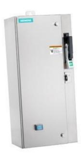
Non-reversing motor starter, Size 1 3/4, Three phase full voltage, Solid-state overload relay, OLRelay amp range 10-40a, 550/575 600 50/60HZ coil, Combination type, 60Amp non-fused disconnect Encl NEMA type 4X 304 S-steel Water/dust tight noncorrosive, Standard width enclosure
