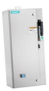
Non-reversing motor starter, Size 1 3/4, Three phase full voltage, Solid-state overload relay, OLRelay amp range 10-40a, 110V 50HZ / 120V 60HZ coil, Combination type, 60Amp non-fused disconnect Encl NEMA type 4X 304 S-steel Water/dust tight noncorrosive, Standard width enclosure
