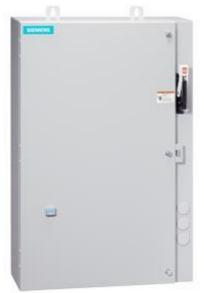
Non-reversing motor starter Size 2 Three phase full voltage Amb compensate bimetal OLrelay Contactor amp rating 45Amp 24Vdc coil Combination type 60Amp fusible disconnect 60Amp / 600V fuse clip Enclosure NEMA type 4/12 Water/dust tight weather proof Extra-wide enclosure
