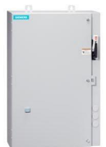
Non-reversing motor starter Size 0 Three phase full voltage Amb compensate bimetal OLrelay Contactor amp rating 18Amp 208VAC 60HZ coil Combination type 3Amp circuit breaker Enclosure NEMA type 4/12 Water/dust tight for outdoors Extra-wide enclosure
