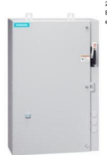
Non-reversing motor starter Size 0 Three phase full voltage Amb compensate bimetal OLrelay Contactor amp rating 18Amp 190-220/220-240V 50/60HZ coil Combination type 3Amp circuit breaker Enclosure NEMA type 4/12 Water/dust tight for outdoors Extra-wide enclosure
