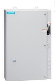
Non-reversing motor starter Size 0 Three phase full voltage Amb compensate bimetal OLrelay Contactor amp rating 18Amp 240V 50HZ / 277V 60HZ coil Combination type 3Amp circuit breaker Enclosure NEMA type 4/12 Water/dust tight for outdoors Extra-wide enclosure
