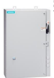
Non-reversing motor starter Size 0 Three phase full voltage Amb compensate bimetal OLrelay Contactor amp rating 18Amp 240V 50HZ / 277V 60HZ coil Combination type 10Amp circuit breaker Enclosure NEMA type 4/12 Water/dust tight for outdoors Extra-wide enclosure
