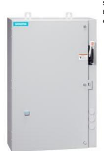
Non-reversing motor starter Size 0 Three phase full voltage Amb compensate bimetal OLrelay Contactor amp rating 18Amp 110V 50HZ / 120V 60HZ coil Combination type 25Amp circuit breaker Enclosure NEMA type 4/12 Water/dust tight for outdoors Extra-wide enclosure
