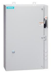
Non-reversing motor starter Size 0 Three phase full voltage Amb compensate bimetal OLrelay Contactor amp rating 18Amp 190-220/220-240V 50/60HZ coil Combination type 25Amp circuit breaker Enclosure NEMA type 4/12 Water/dust tight for outdoors Extra-wide enclosure
