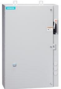
Non-reversing motor starter Size 0 Three phase full voltage Amb compensate bimetal OLrelay Contactor amp rating 18Amp 110-120/220-240VAC 60HZ coil Combination type 3Amp circuit breaker Encl NEMA type 4X 304 S-steel Water/dust tight noncorrosive Extrawide enclosure
