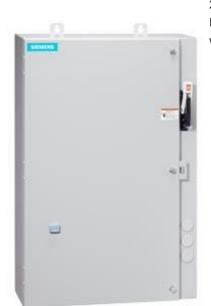
Non-reversing motor starter Size 0 Three phase full voltage Amb compensate bimetal OLrelay Contactor amp rating 18Amp 220-240/440-480VAC 60HZ coil Combination type 3Amp circuit breaker Encl NEMA type 4X 304 S-steel Water/dust tight noncorrosive Extrawide enclosure
