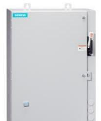
Non-reversing motor starter Size 0 Three phase full voltage Amb compensate bimetal OLrelay Contactor amp rating 18Amp 208VAC 60HZ coil Combination type 3Amp circuit breaker Encl NEMA type 4X 304 S-steel Water/dust tight noncorrosive Extra-wide enclosure
