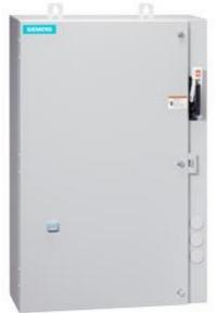
Non-reversing motor starter Size 0 Three phase full voltage Amb compensate bimetal OLrelay Contactor amp rating 18Amp 110V 50HZ / 120V 60HZ coil Combination type 3Amp circuit breaker Encl NEMA type 4X 304 S-steel Water/dust tight noncorrosive Extra-wide enclosure
