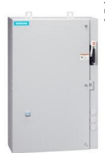
Non-reversing motor starter Size 0 Three phase full voltage Amb compensate bimetal OLrelay Contactor amp rating 18Amp 380-440/440-480V 50/60HZ coil Combination type 3Amp circuit breaker Encl NEMA type 4X 304 S-steel Water/dust tight noncorrosive Extrawide enclosure
