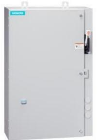
Non-reversing motor starter Size 0 Three phase full voltage Amb compensate bimetal OLrelay Contactor amp rating 18Amp 240V 50HZ / 277V 60HZ coil Combination type 3Amp circuit breaker Encl NEMA type 4X 304 S-steel Water/dust tight noncorrosive Extra-wide enclosure
