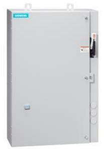
Non-reversing motor starter Size 0 Three phase full voltage Amb compensate bimetal OLrelay Contactor amp rating 18Amp 110-120/220-240VAC 60HZ coil Combination type 10Amp circuit breaker Encl NEMA type 4X 304 S-steel Water/dust tight noncorrosive Extrawide enclosure
