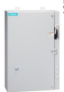
Non-reversing motor starter Size 0 Three phase full voltage Amb compensate bimetal OLrelay Contactor amp rating 18Amp 220-240/440-480VAC 60HZ coil Combination type 10Amp circuit breaker Encl NEMA type 4X 304 S-steel Water/dust tight noncorrosive Extrawide enclosure
