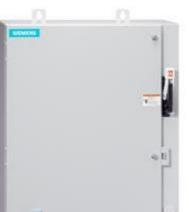
Non-reversing motor starter Size 0 Three phase full voltage Amb compensate bimetal OLrelay Contactor amp rating 18Amp 208VAC 60HZ coil Combination type 10Amp circuit breaker Encl NEMA type 4X 304 S-steel Water/dust tight noncorrosive Extra-wide enclosure
