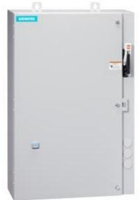
Non-reversing motor starter Size 0 Three phase full voltage Amb compensate bimetal OLrelay Contactor amp rating 18Amp 550/575-600 50/60HZ coil Combination type 10Amp circuit breaker Encl NEMA type 4X 304 S-steel Water/dust tight noncorrosive Extra-wide enclosure
