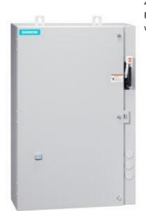
Non-reversing motor starter Size 0 Three phase full voltage Amb compensate bimetal OLrelay Contactor amp rating 18Amp 380-440/440-480V 50/60HZ coil Combination type 10Amp circuit breaker Encl NEMA type 4X 304 S-steel Water/dust tight noncorrosive Extrawide enclosure
