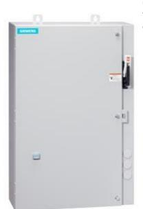
Non-reversing motor starter Size 0 Three phase full voltage Amb compensate bimetal OLrelay Contactor amp rating 18Amp 24VAC 50-60HZ coil Combination type 10Amp circuit breaker Encl NEMA type 4X 304 S-steel Water/dust tight noncorrosive Extra-wide enclosure
