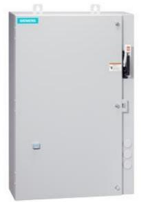
Non-reversing motor starter Size 0 Three phase full voltage Amb compensate bimetal OLrelay Contactor amp rating 18Amp 240V 50HZ / 277V 60HZ coil Combination type 10Amp circuit breaker Encl NEMA type 4X 304 S-steel Water/dust tight noncorrosive Extra-wide enclosure
