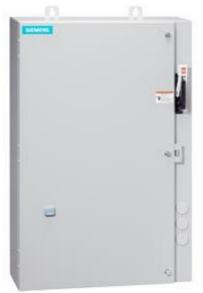
Non-reversing motor starter Size 0 Three phase full voltage Amb compensate bimetal OLrelay Contactor amp rating 18Amp 110-120/220-240VAC 60HZ coil Combination type 25Amp circuit breaker Encl NEMA type 4X 304 S-steel Water/dust tight noncorrosive Extrawide enclosure
