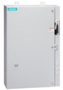
Non-reversing motor starter Size 0 Three phase full voltage Amb compensate bimetal OLrelay Contactor amp rating 18Amp 220-240/440-480VAC 60HZ coil Combination type 25Amp circuit breaker Encl NEMA type 4X 304 S-steel Water/dust tight noncorrosive Extrawide enclosure
