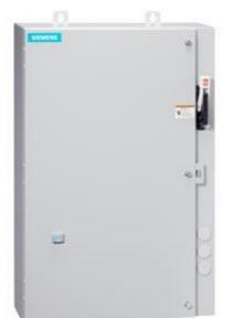
Non-reversing motor starter Size 0 Three phase full voltage Amb compensate bimetal OLrelay Contactor amp rating 18Amp 208VAC 60HZ coil Combination type 25Amp circuit breaker Encl NEMA type 4X 304 S-steel Water/dust tight noncorrosive Extra-wide enclosure
