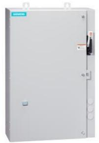
Non-reversing motor starter Size 0 Three phase full voltage Amb compensate bimetal OLrelay Contactor amp rating 18Amp 550/575-600 50/60HZ coil Combination type 25Amp circuit breaker Encl NEMA type 4X 304 S-steel Water/dust tight noncorrosive Extra-wide enclosure
